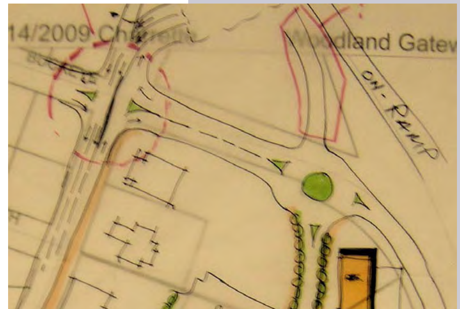
Traffic circulation concept for Woodland's Gateway District, showing a reconfigured Buckeye/Goerig intersection and a round-about as part of new access roads into the Gateway District.
