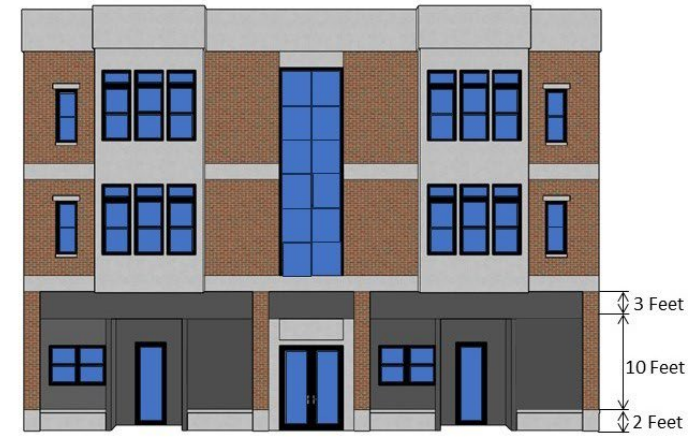
Unacceptable amount of ground floor window transparency (less than fifty percent minimum).
