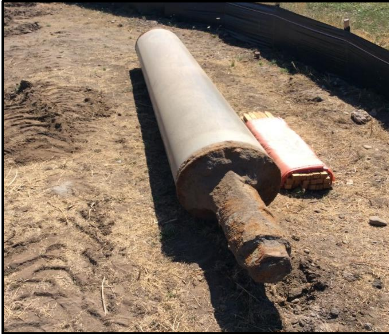
ROLLER IS FROM GEORGIA GRANITE MEASUREMENTS: 24" DIAMETER 12' LONG
