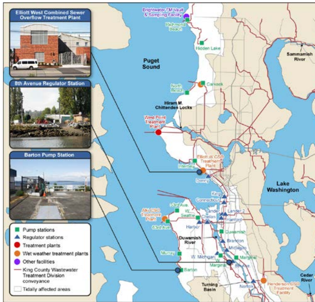
King County Wastewater Treatment Division Facilities Potentially Vulnerable to Sea Level Rise Source: US GAO Report: Climate Change: Future Federal Adaptation Efforts Could Better Support Local Infrastructure Decision Makers
